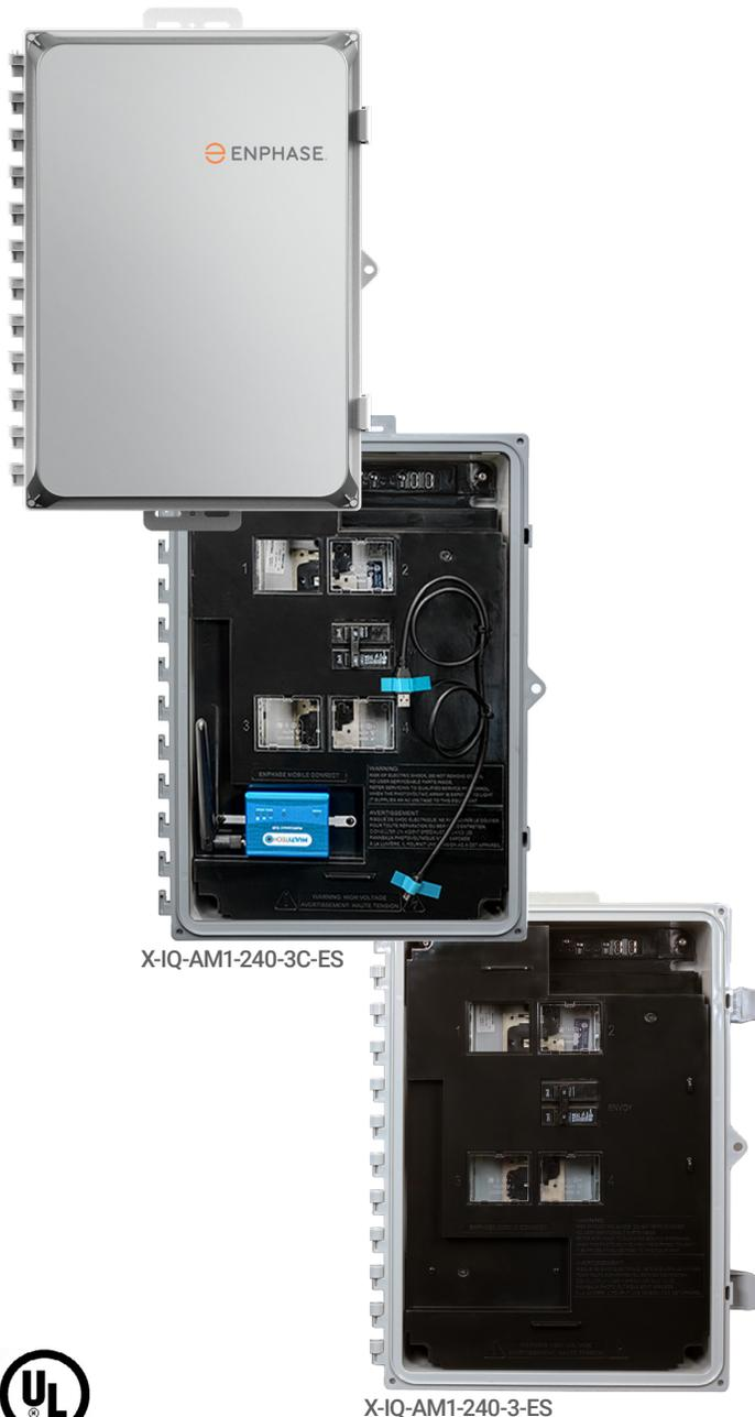
The **Enphase IQ Combiner 3-ES/3C-ES** with Enphase IQ Gateway and integrated LTE-M1 cell modem (included only with IQ Combiner 3C-ES) consolidates interconnection equipment into a single enclosure and streamlines PV and storage installations by providing a consistent, pre-wired solution for residential applications. It offers up to four 2-pole input circuits and Eaton BR series busbar assembly.
